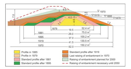
Fig. 4. Rise of the embankments (compiled by Schweitzer, F. after Vágás, I. 1982)
